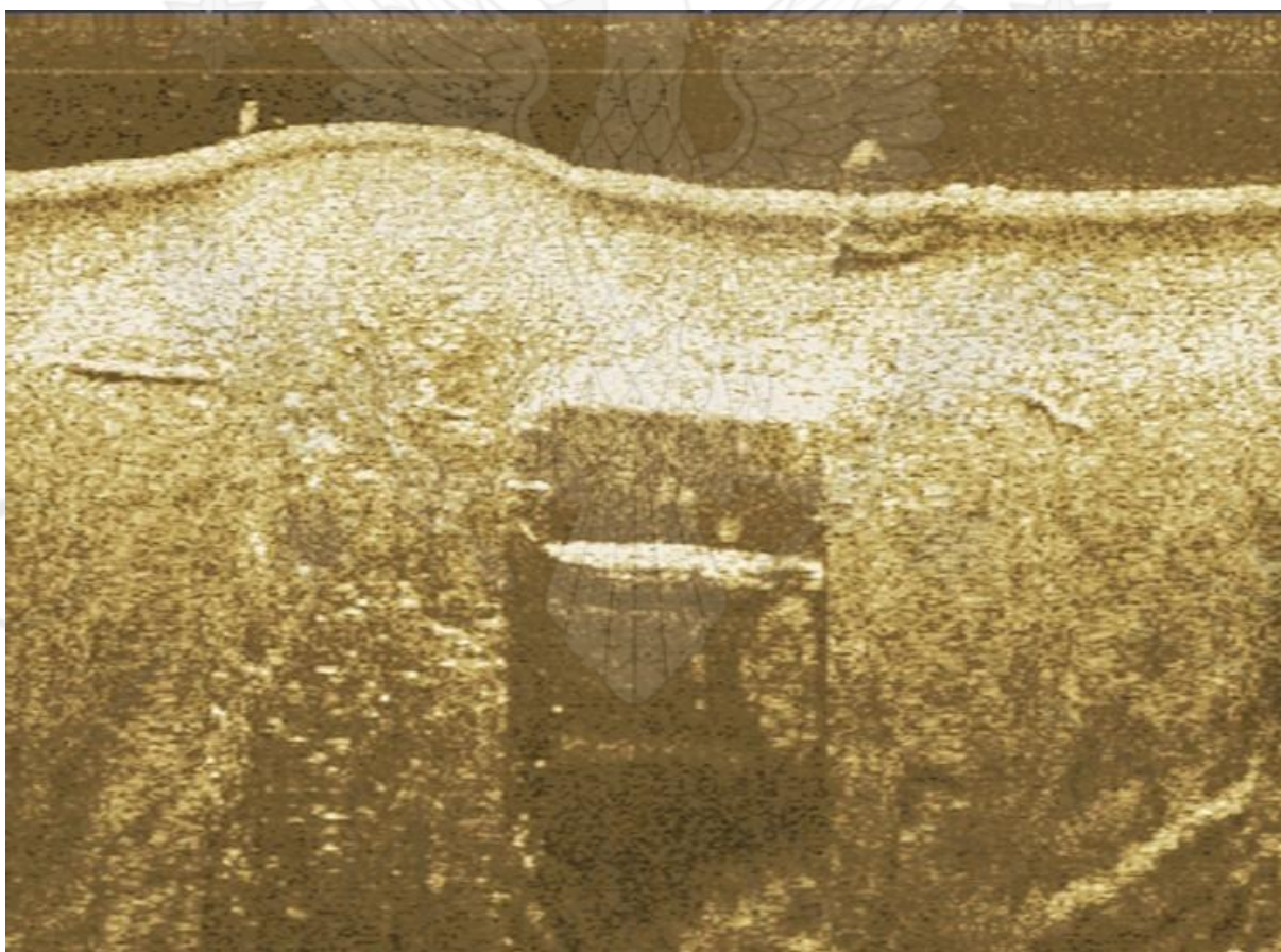
Fig. 6 – The wreck as seen on side-scan sonar image (image by: P. Maliński)
